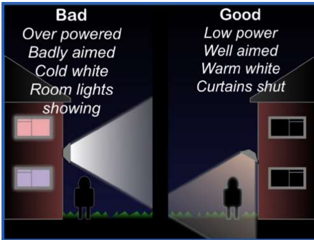
Diagram showing the impact of shielded light fittings on commercial premises. Courtesy Commission for Dark Skies
