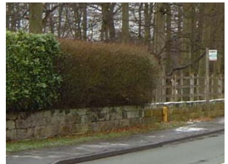
Three courses of stone blocks, natural stone kerb adjacent to the footway.
