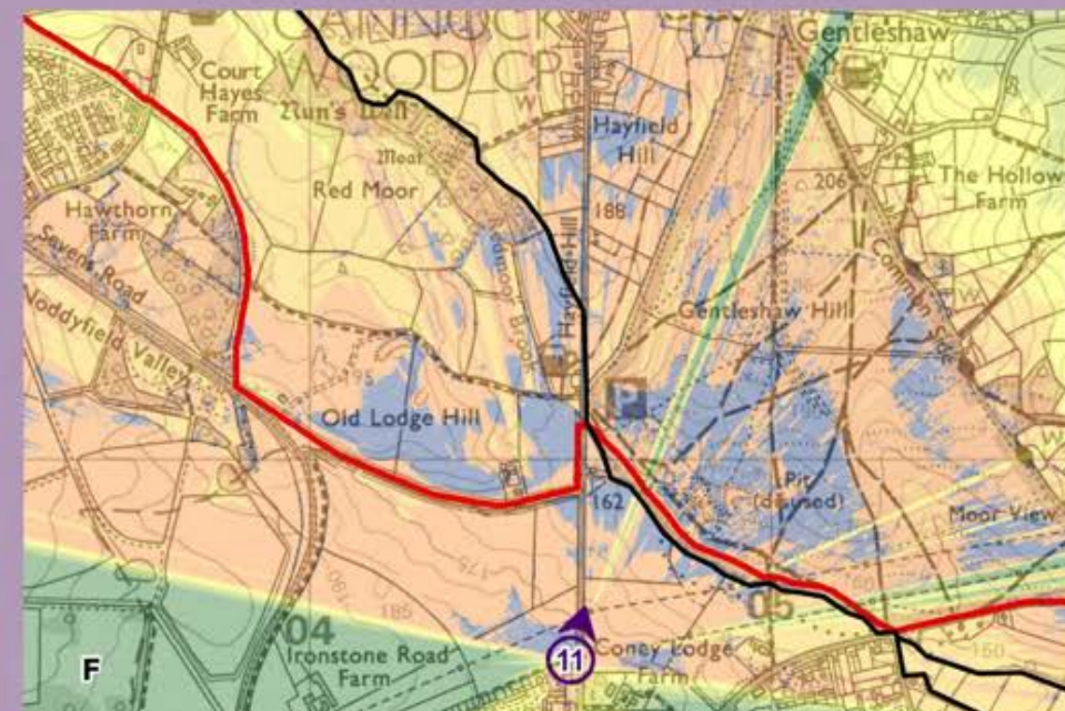
The electricity transmission tower / pylon is represented as a solid visual barrier within the ZTV output, detracting from the data's objectivity.
